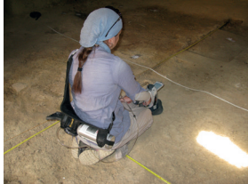
Analysing floor surfaces for geochemical elements in a modern traditional village
